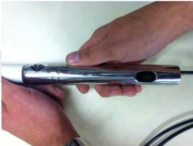
19. Place the solid rubber hole-plug that came with the antenna into the hole.
