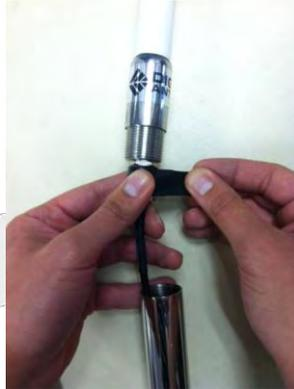
18. Once the tape is applied, slide the tube up to the antenna and screw the tube on finger-tight.
