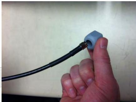
10. Push the cable through the Cord Grip into the enclosure.
