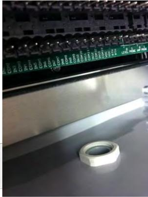
9. Run the smaller end of the coax cable through the bushing nut.
