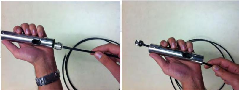
16. Attach the coax cable to the antenna (**finger-tight only!**)
