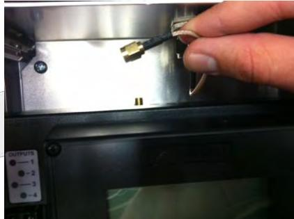
2. Remove the Phantom Antenna from the Enclosure by unscrewing the nut with a wrench.
