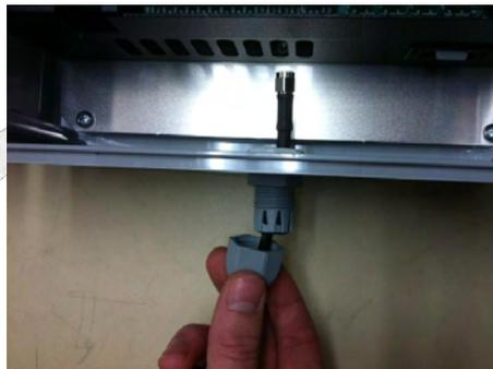
11. Smoothly route the cable around the Unit and attach the cable to the Radio.
