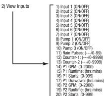
**Key:** (range or options; 1) Input 1 (ON/OFF) default) 2) Input 2 (ON/OFF) 3) Input 3 (ON/OFF)
