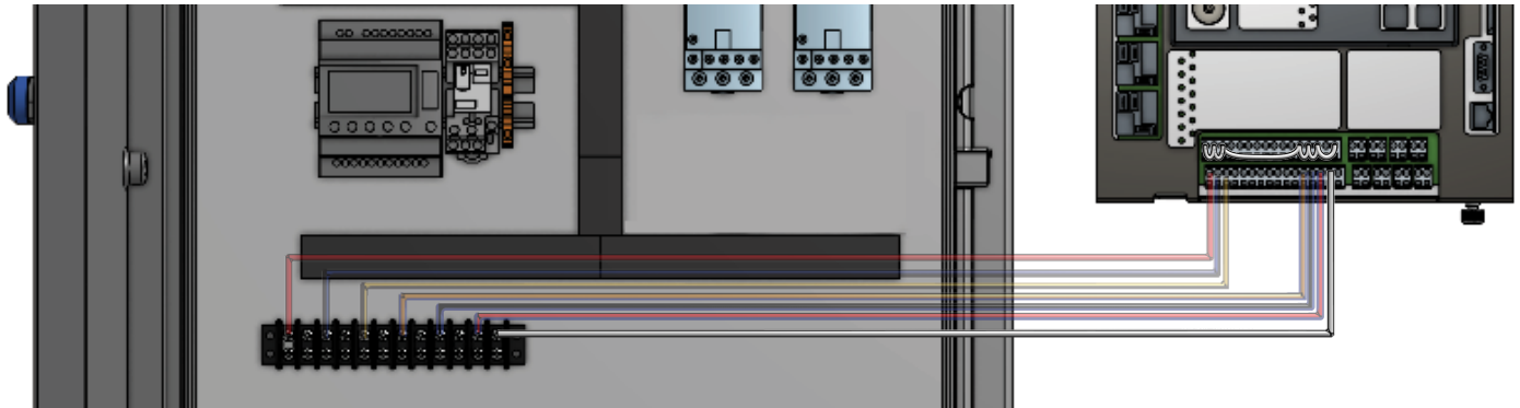
Fig. 8: Terminal Strip for Digital Inputs Neutral Wire
