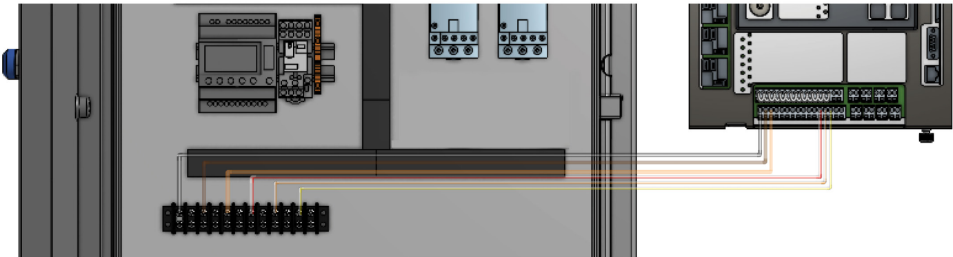
Fig. 8: Terminal Strip for Digital Inputs Neutral Wire
