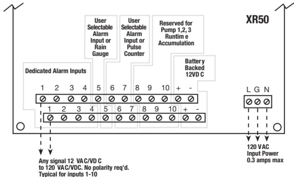
Note: Different voltages can be applied to different input channels as needed (I.E. Don't all have to be the same)
